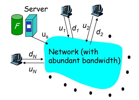
Time to distribute Fto N clients using =  $d_{cs} = max \{ NF/u_{s}, F/min(d_i) \}$ client/server approach increases linearly in N (for large N) 2: Application Layer 17
